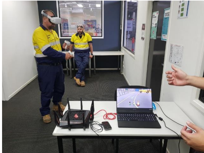
Figure 13 Example hardware setup at RTO. Note the lack of tether to the headset and high-speed internet router (crown like device on the table) streaming the VR experience to the headset.
