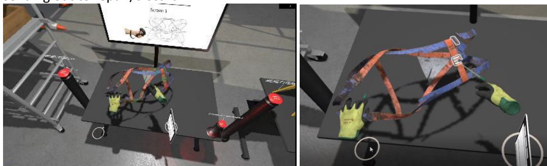
Figure 6 Images showing the harness examination process at the station (left). On the right we see the trainee highlighting and selecting the broken D-Ring (right).
